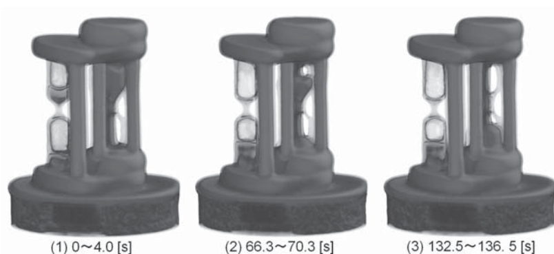
Figure 2: 4D-CT sample image (240 projection numbers; 60 fps; 0.25 revolution per second).
