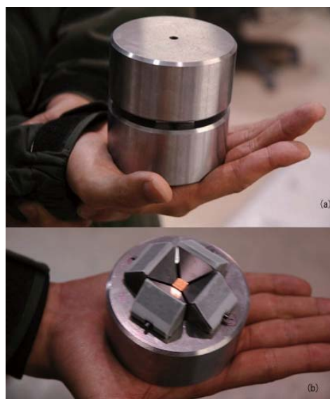
Fig. 1. Downsized Cubic anvil type high pressure cell optimized for neutron scattering experiments
