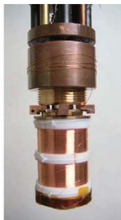
Fig. 1. Pressure cell together with the AC susceptibility coil.
