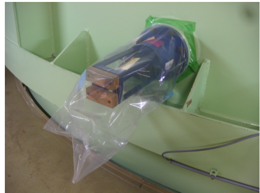
Fig. 3. Collecting leaking \text{SF}_6 gas in a plastic bag for searching leak spots.
