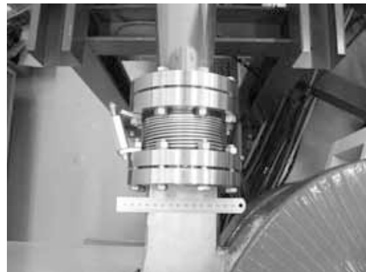
Fig.4 The bellow pressed by the vacuum chamber of the electromagnet, it caused the vacuum break.
