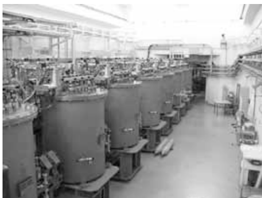
Fig. 3 Schematic view of cryostats of the superconducting booster. The back side of this picture is joint of the buildings.
